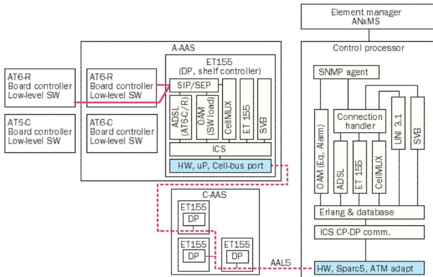
Figure 8 Software partitioning in an ANx-DSL system.
