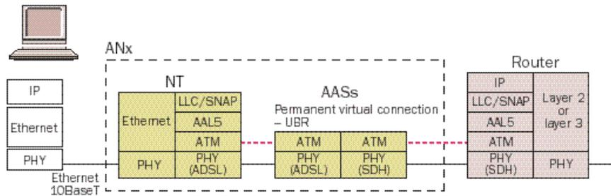
users of a high-capacity ANx solution. ANx-DSL provides high-speed transport for IP-format packets, regardless of whether a user is connected to a 10BaseT interface or to an ATM-F 25.6 interface.
